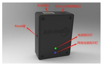
Reset button / RJ45 network port / MicroUSB power port /
